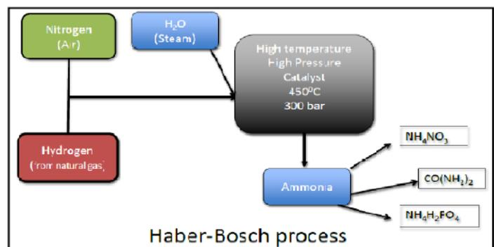
Figure. 2 Synthetic fertilizer production process
