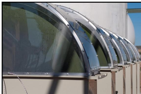
**Figure 1:** ALGADISK pilot reactor installed at Biogas Fuel Cell site in Almazan, Spain
